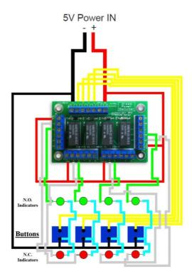
Figure 1 - Connection Diagram
