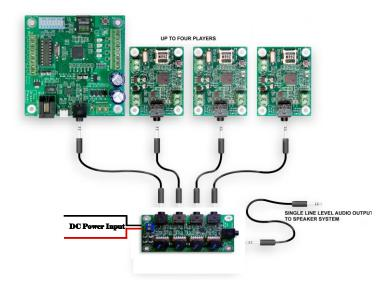
**Figure 1 - Connection Diagram**
